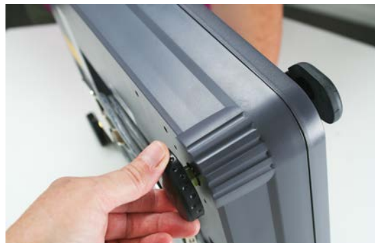
Figure 2-4. Adjust the Scale Base Feet
