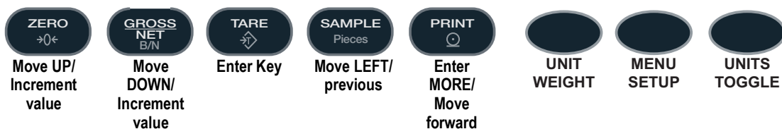
Figure 3-2. Front Panel Key Functions in Menu Mode
