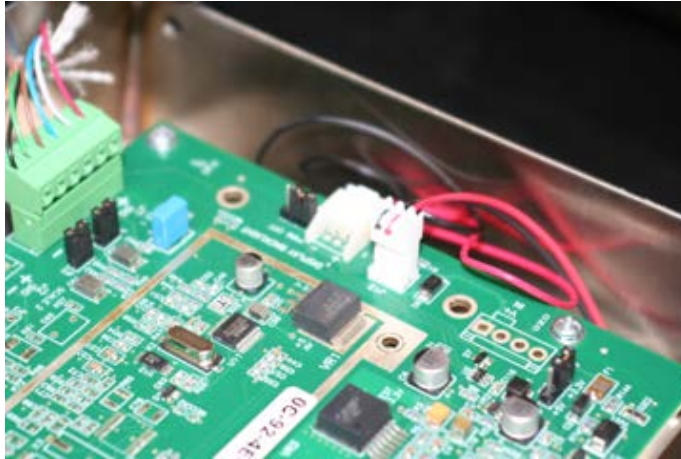
Figure 2-14. Connect Power Plug onto J12 on CPU Board
