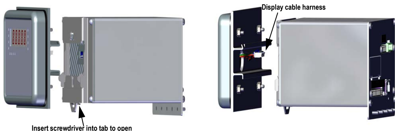
Figure 2-4. Install Controller Assembly
