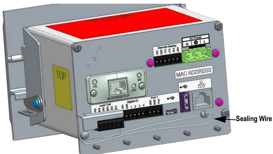
Figure 2-27. Install Sealing Wire
