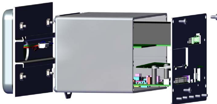
Figure 2-9. Remove Controller Assembly Backplate
